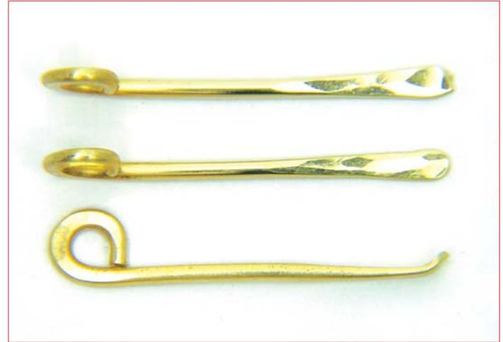
2. Flatten the pointed end of the wire into a tapered tongue shape, forging about half the remaining wire length (top). Use a flat file to shape the wire's tip and sanding pad to round it smoothly (middle). Bend the tip of the flattened wire 45 degrees upward to create a 'ski tip' to serve as the catch ring's gateway (bottom).
