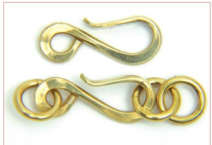
4. Lay the S-clasp on the anvil and forge the remaining round wire between the two loops (top). Adjust the large loop's gateway to allow the snug passage of a 15-gauge catch ring, assembled 1+1 for bracelet length adjustability, and a third catch ring through the clasp's small loop (bottom).
